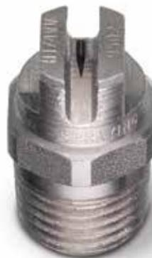
**VeeJet® nozzles** produce a thin, tapered-edge, rectangular spray pattern with medium sized drops and higher impact. Positioned to the side of the rail cars, the higher impact spray penetrates the falling iron ore and provides effective dust control.
