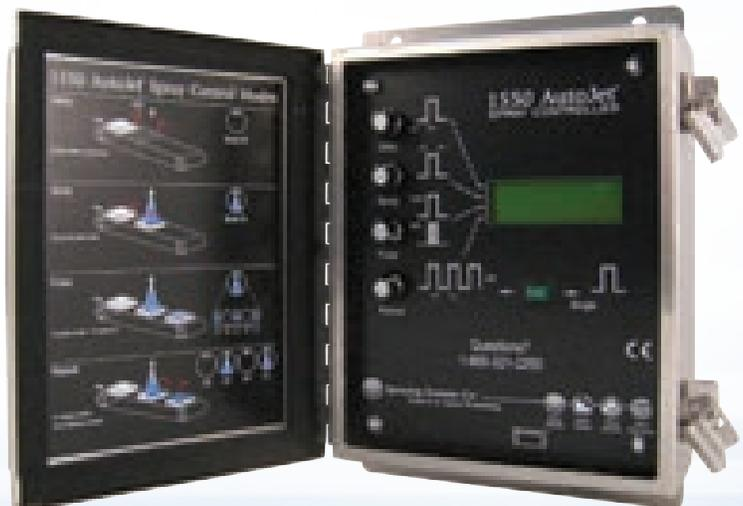
**Modular Spray System** provides easy control of nozzles and cycle times up to 10,000 cycles per minute
