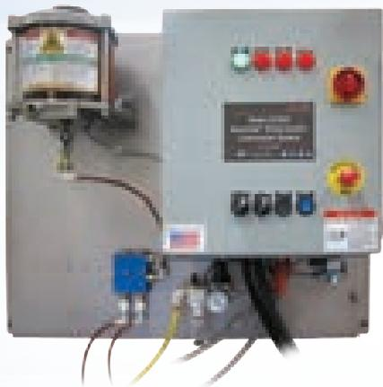
The patent-pending Model 52200 AutoJet Electrostatic Lubrication System improves chain lubrication while greatly reducing oil consumption and conveyor downtime. The system is built around an AutoJet Spray Controller, electrostatic spray nozzles, a 16 liter (4.2 gallon) oil reservoir and a pressure regulator/filter/pressure switch. The system offers real-time monitoring of system parameters, including automated warning and alarm functions.
