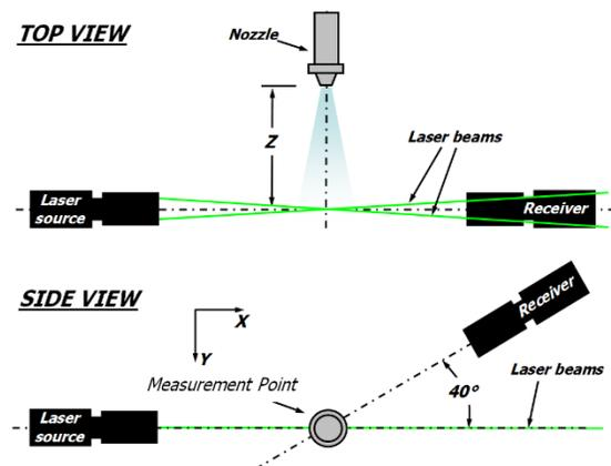
Figure 1. Illustration of PDI layout for drop size and velocity data acquisition.
