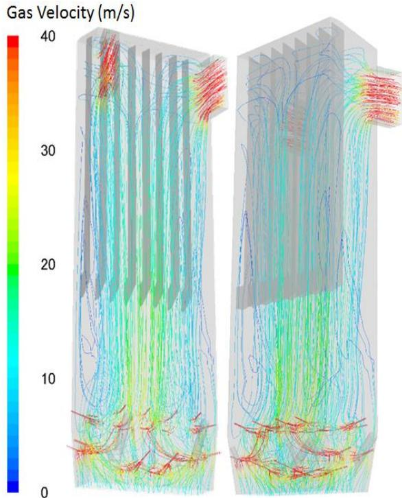
**Figure 6.** Gas Phase Pathlines Colored by Gas Velocity in CFB Boiler
