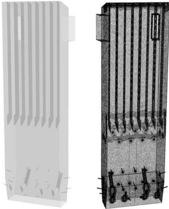
**Figure 4.** 3D Circulating Fluidized Bed Boiler Geometry for CFD
