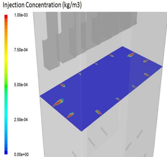
**Figure 11.** Contour of Aqueous Ammonia Concentration on the Injection Plane
