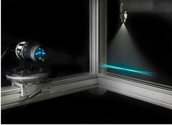
**Figure 2.** Illustration of PDI during experiment.
