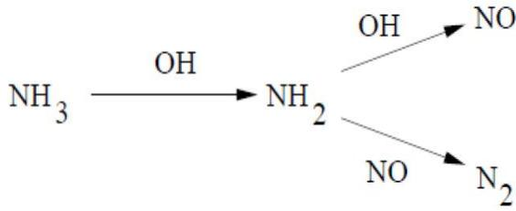
**Figure 5.** Simplified Reaction Mechanism for the SNCR process
