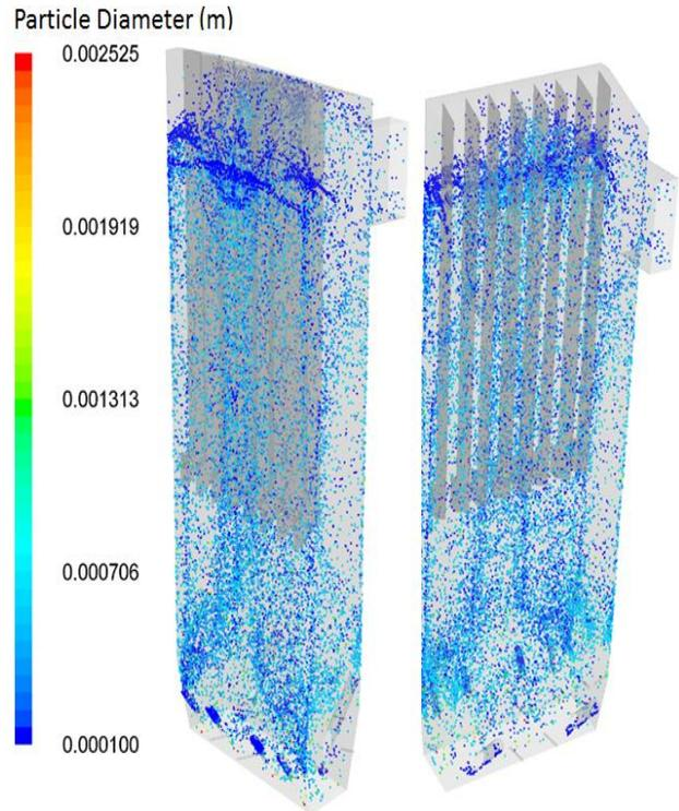
**Figure 7.** Solid Phase Particulate Distribution Colored by Diameter in CFB Boiler
