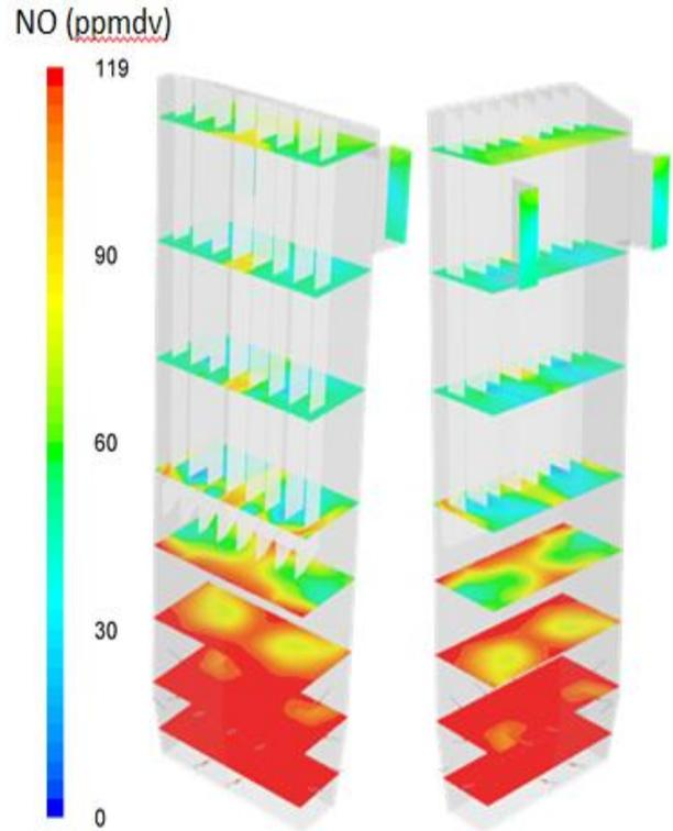
**Figure 12.** Contour of Nitrogen Dioxide Distribution after SNCR
