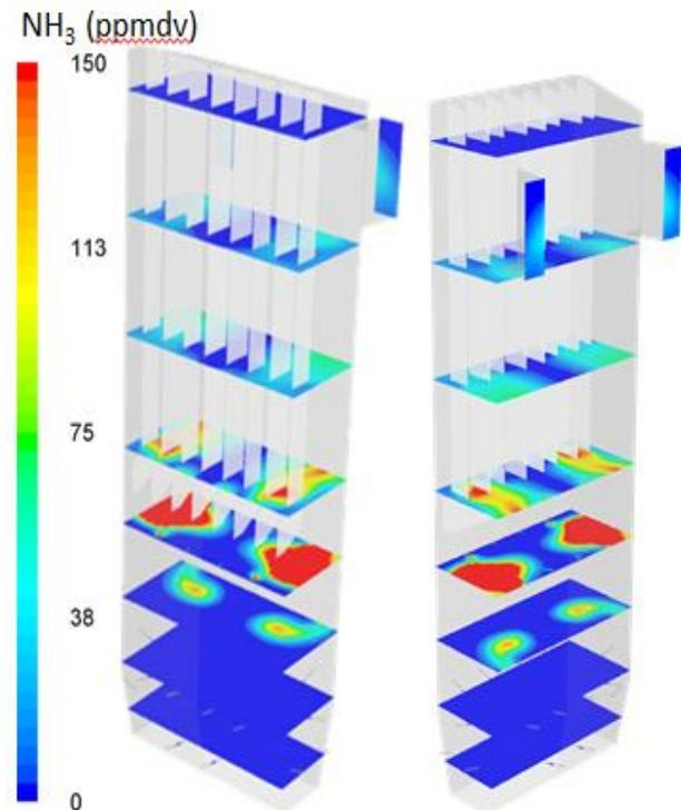
**Figure 13.** Contour of Ammonia Distribution after SNCR
