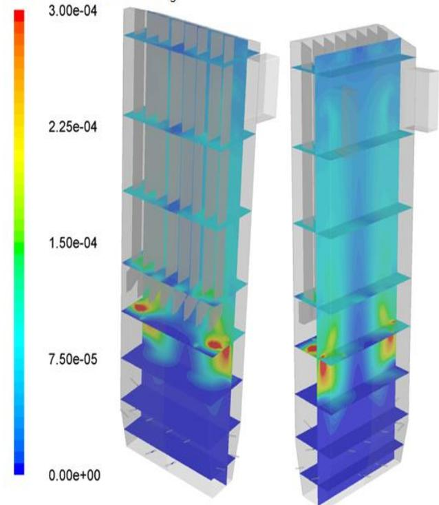
**Figure 10.** Mass Fraction of Vapor Ammonia Evaporated into Gas Phase Species
