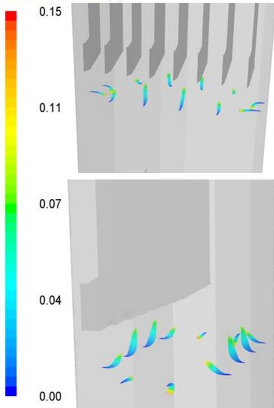
**Figure 9.** Tracked Reagent Droplet Residence Time in Seconds at Injection Points
