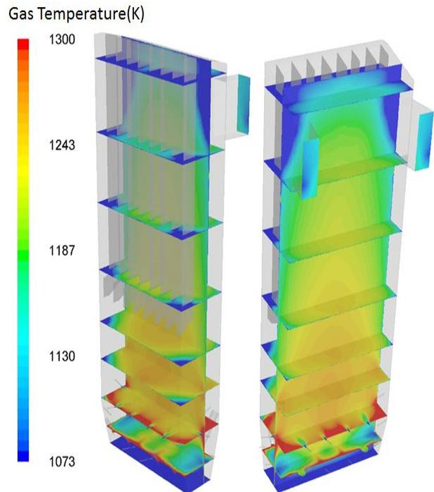
**Figure 8.** Temperature Profile at Various Heights of Gas Phase in the CFB Boiler
