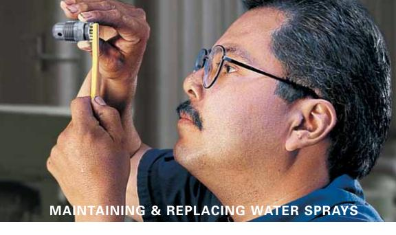
**Nozzle orifices are precision engineered. Be careful to avoid damage when cleaning.** Use cleaning tools that are significantly softer than the material of the sprays like a toothbrush or toothpick. Never clean the orifice with metal objects.
